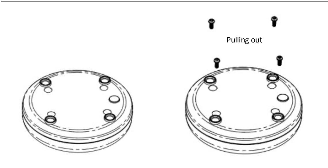
3. Take the front cover out and pull out the cell battery as the picture.
