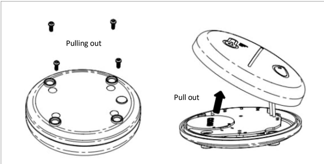
4. Take the cell battery out using a screw driver for pulling out the cell battery as the picture.
