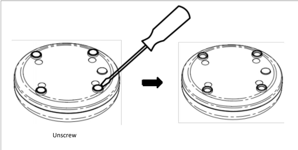
2. Pulling out the screws from the plastic casing to change the battery.
