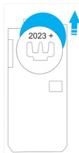
15. Slide a new CR2032 battery into the battery casing, making sure that the polarity is correct.
