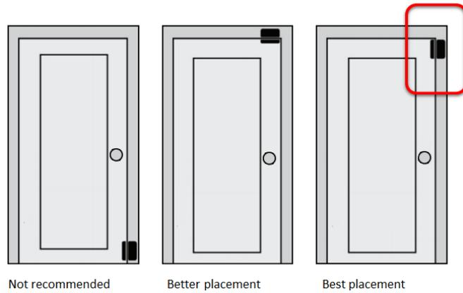
The sensors and magnet each have a slightly engraved line. This line denotes where the sensors align to function properly. If the sensor and magnet, when together/closed, do not line up correctly, the sensor will not report correctly. See Figure 2.
