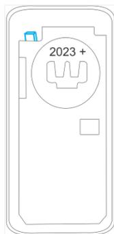
13. Press and hold the tab away from the circuit board, and then turn the sensor over.
